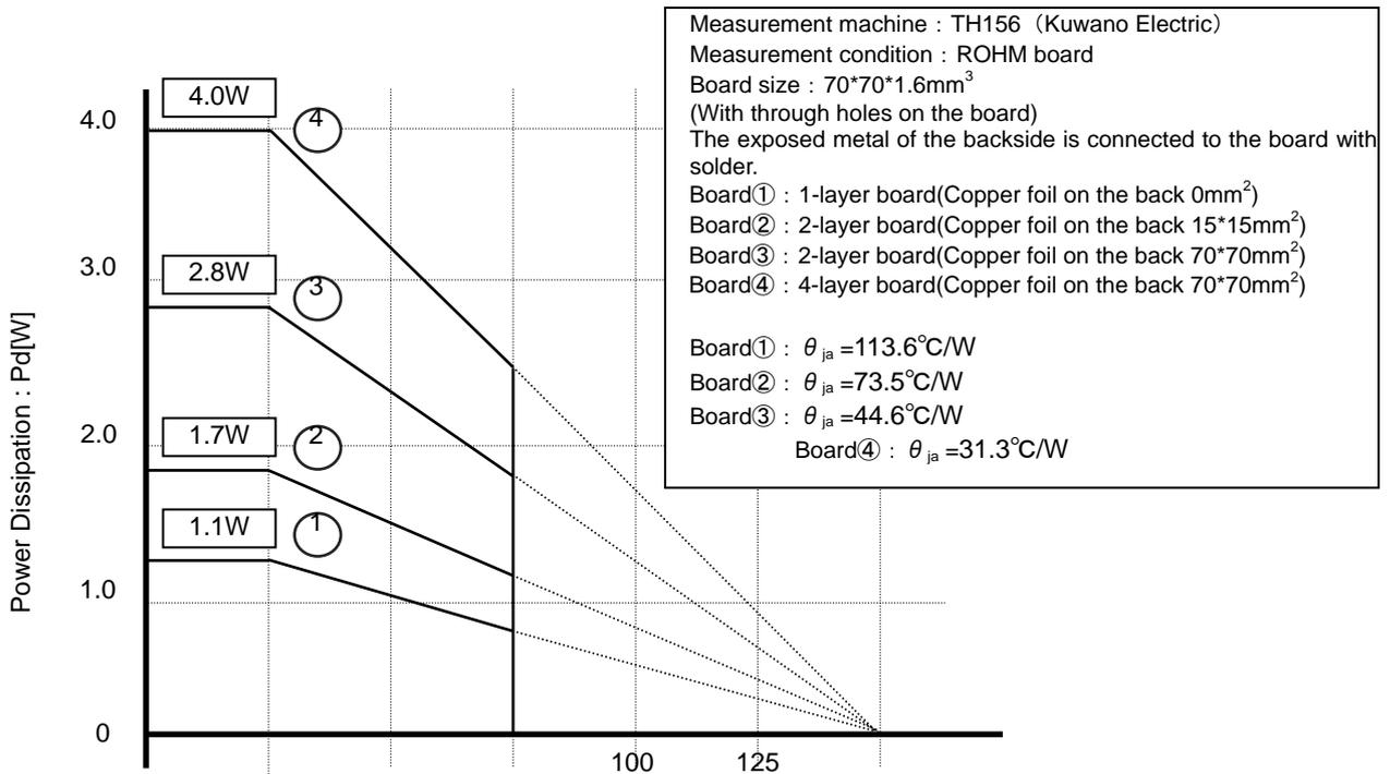
Fig.2 HTSSOP-B24 Derating curve
